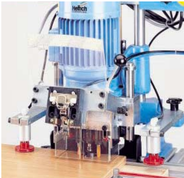
5 Drilling process is initiated by pressing the foot pedal.
