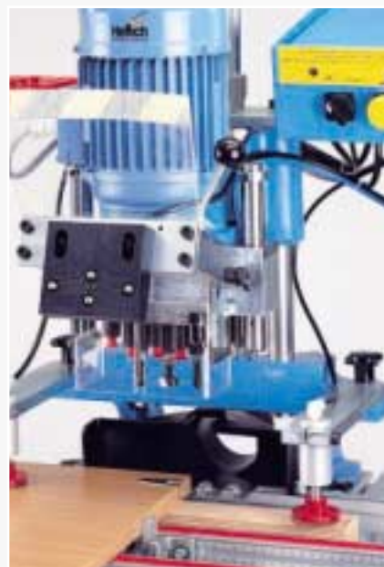
9 Connecting fitting is perfectly seated in the shelf, release the hold-down clamps (yellow button) ...
