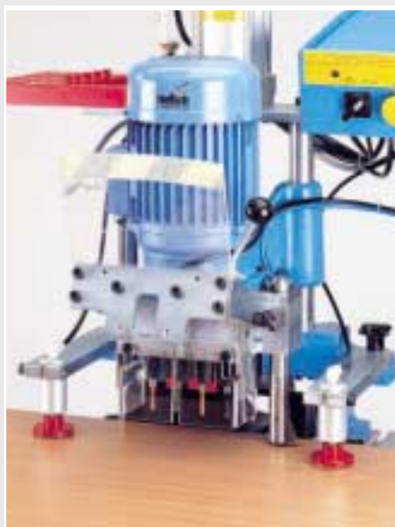
Hole line boring in System 32 with the integrated indexing stop system
