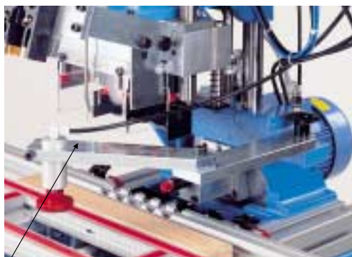
Extension arm for hold-down clamp, practical in conjunction with ● retrofitted single-spindle horizontal boring unit ● narrow workpieces
