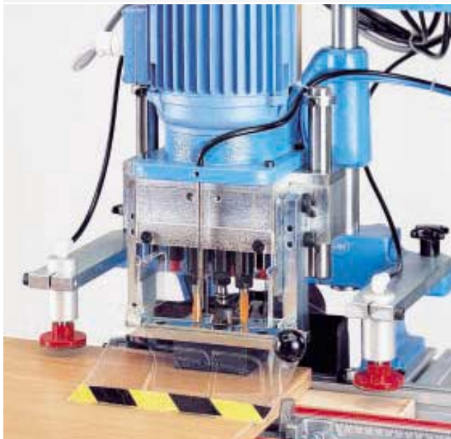
7 Insertion procedure: swing down insertion unit, press foot pedal ... hinge is inserted.
