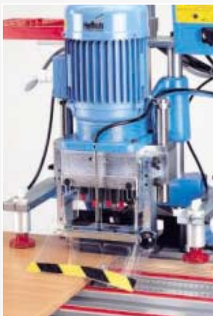
8 Insertion procedure: swing down insertion unit, press foot pedal ... connecting fitting is inserted.
